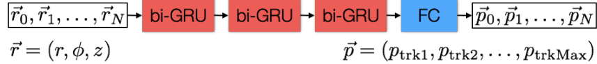
Figure 5: The spacepoint sequence model takes as input the full set of spacepoint measurements in the detector and outputs a track probability assignment matrix.
